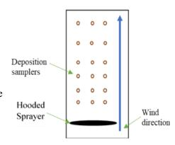
residue analysis to quantify dicamba deposition. Testing conditions are established herein with the express purpose of producing and comparing drift deposition curves between a baseline and a proposed hooded sprayer and are therefore not intended to be representative of field conditions.
